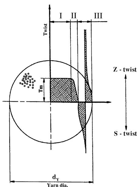
**Figure 1. The rotor spun yarn cross section showing twist distribution**
